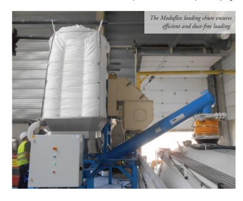
TBMA designed and supplied a customengineered big-bag discharging installation. Key words were high-capacity, ergonomic design, flexibility and minimal dust emission. Also, the system should be able to load two bulk trucks at once.
