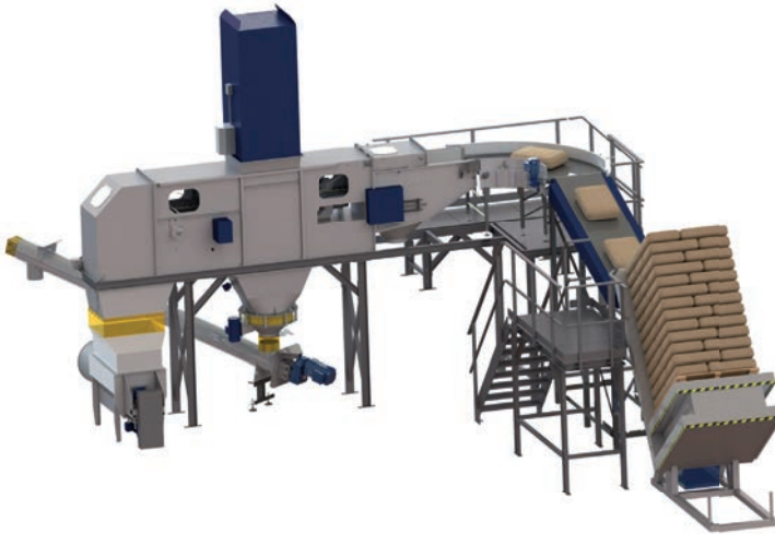
Semi-automatic Galahad machine with lift-tilting table
