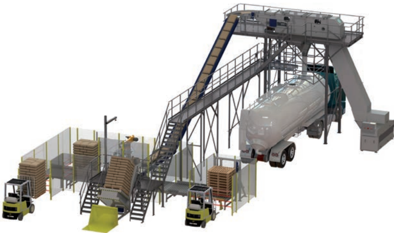
Full-automatic Galahad machine with multi-head robot and additional lift-tilting table.
