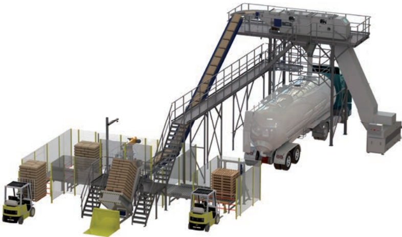
Full-automatic Galahad machine with multi-head robot and additional lift-tilting table.
