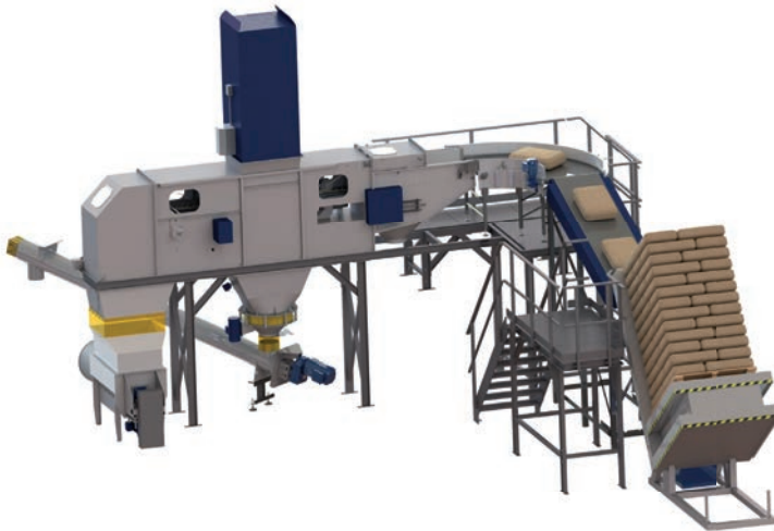
Semi-automatic Galahad machine with lift-tilting table
