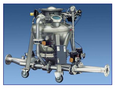
Due to the dense phase conveying principle the pressure in the system will be higher than in a dilute phase system and results in pressures of 1 to 6 bar. Conveying velocities of 1-10 m/s and distances of 500 m or more with capacities up to 100 t/hr can be achieved. The inlet valve, being the only moving part, makes the special designed dense phase "Vackonveyor" suitable for conveying abrasive products and products where no segregation or degradation is allowed...
