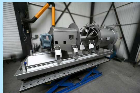
Quickly demountable batch mixer equipped with a rail system and residue collection tray
