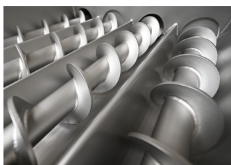
Detail of the multi-screw dosing system for potato flakes
