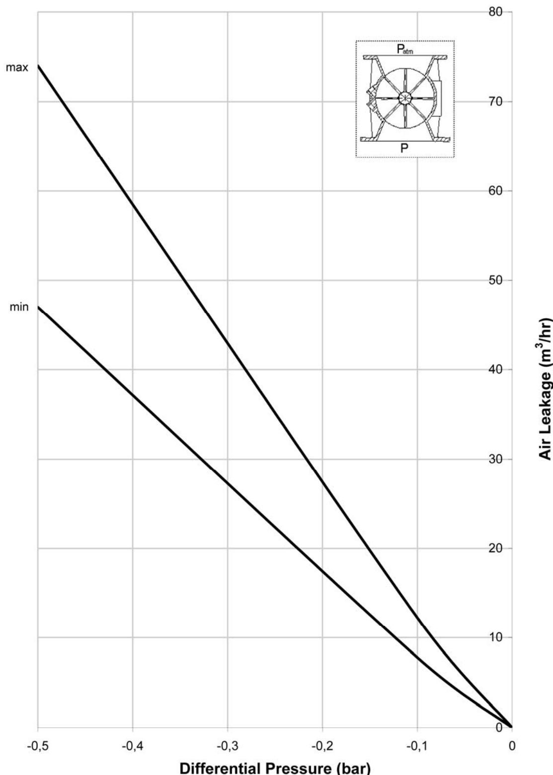
Air leakage indicated is the maximum and minimum value found during testing.
