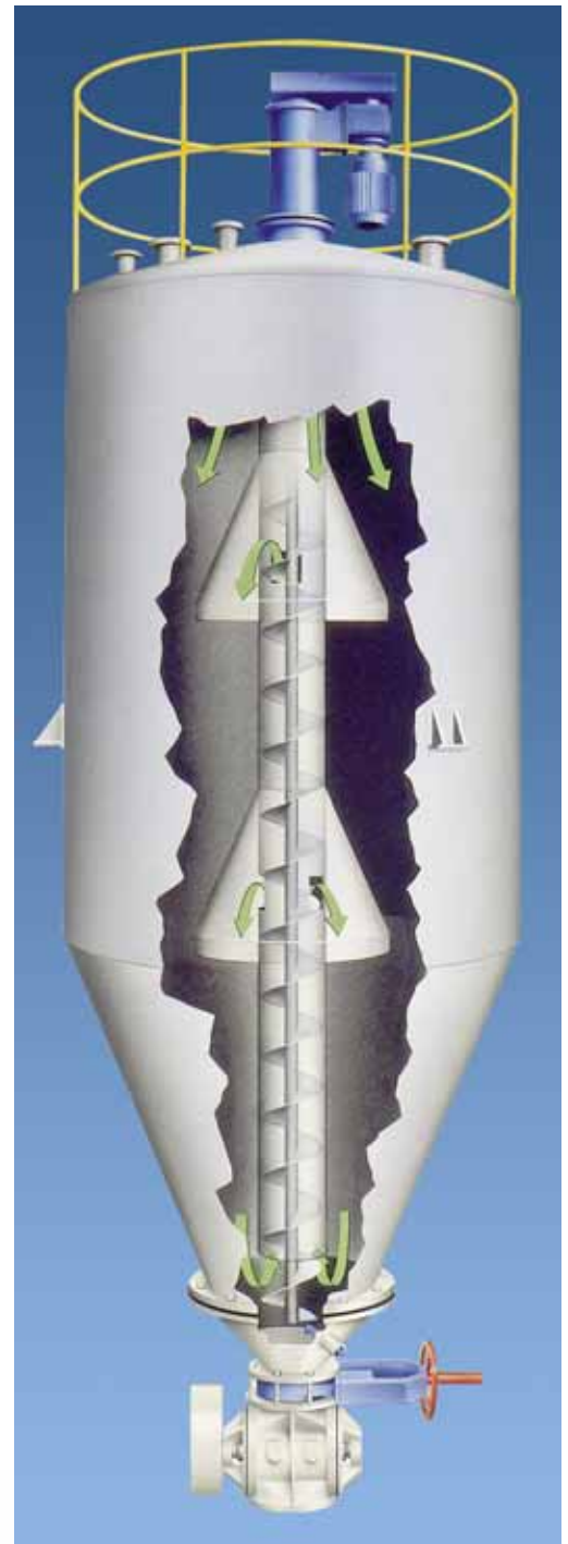
Principle of operation of VRM vertical mixer
