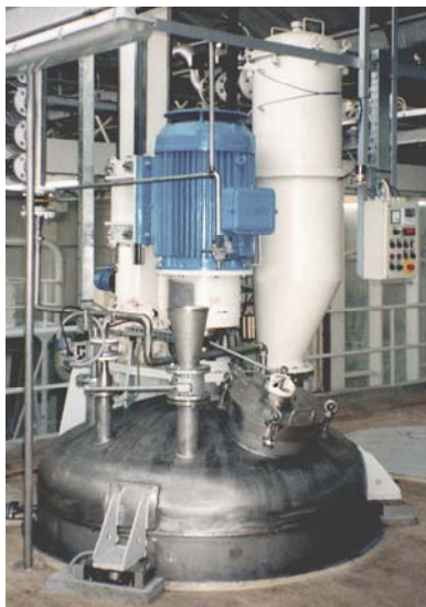
Turbo-Mixer for artificial leather production
